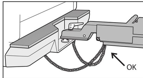
Be sure to leave enough slack in the chains/cables to turn corners without binding; however, note that excessive slack will allow the chains/cables to drag on the ground.
