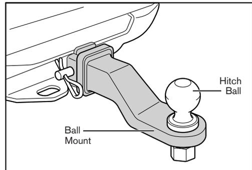
The diameter of the hitch ball shank must be matched to the ball mount hole diameter. The shank should be no more than 1<sup>1</sup>/<sub>16</sub>” smaller than the hole.
