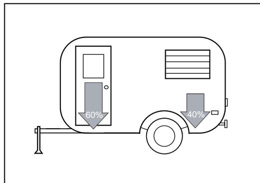
With this in mind, proper loading is extremely important. When loading a trailer, 60% of the total cargo weight should be positioned in the front portion of the trailer and 40% in the back. Then the load should be adjusted until the proper tongue load ratio is achieved.
