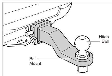
The diameter of the hitch ball shank must be matched to the ball mount hole diameter. The shank should be no more than 1/16” smaller than the hole. To keep the hitch ball in top condition, a simple maintenance routine is recommended. Coating it with light grease will minimize wear of both the coupler and hitch ball. Also, by removing the hitch ball when not towing, or by protecting it with a special cover, you will help prevent rust from forming on it.
