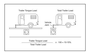
the location of the trailer jack is rearward of the trailer tongue and will not give you an accurate measurement of the true tongue load. Make sure the vehicle jack is placed directly under the trailer tongue coupler, and the tongue is set at the height/level of the tow vehicle hitch.
