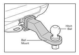
Like ball mounts, hitch balls are available in a number of weight capacities and sizes. Always make sure the hitch ball selected has the proper shank diameter and weight rating for the ball mount as well as the coupler on your
