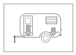
With this in mind, proper loading is extremely important. When loading a trailer, 60% of the total cargo weight should be positioned in the front portion of the trailer and 40% in the back. Then the load should be adjusted until the proper tongue load ratio is achieved.
