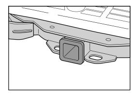
**Clamp-On Bumper Hitch** – This is a temporary hitch that clamps onto the bumper assembly. **DO NOT USE** this type of hitch on any Infiniti vehicle because using it may result in the trailer separating from the towing vehicle; this can cause death or serious injury. Use of this type of hitch can also damage the towing vehicle.
