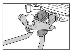
**NOTE** – A weight-distributing hitch system may affect the operation of trailer surge brakes. If you are considering use of a weight-distributing hitch system with a surge brake-equipped trailer, check with the surge brake, hitch, or trailer manufacturer to determine if and how this can be done. Follow the instructions provided by the manufacturer for installing and using the weight-distributing hitch system.
