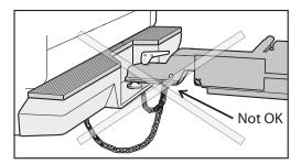
To avoid damage to the bumper and chains/cables when making a sharp turn, do not attach the chains/cables too close to the coupler. Consult your trailer manufacturer for the proper location of the chain/cable attachment to the trailer.
