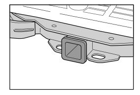
Clamp-On Bumper Hitch – This is a temporary hitch that clamps onto the bumper assembly. DO NOT USE this type of hitch on any Infiniti vehicle because using it may result in the trailer separating from the towing vehicle; this can cause death or serious injury. Use of this type of hitch can also damage the towing vehicle.
