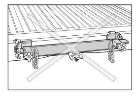
Weight-Distributing Hitch System – This type of system uses a "load-leveling" or "equalizing" hitch. The weight-distributing feature helps shift the trailer tongue weight to all trailer tires and the tow vehicle front tires.
