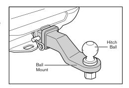
trailer. Using a  $1^7/8$ " hitch ball in a 2" coupler, for example, could result in the trailer separating from the tow vehicle.
