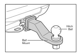
trailer. Using a  $1^7/8$ " hitch ball in a 2" coupler, for example, could result in the trailer separating from the tow vehicle.
