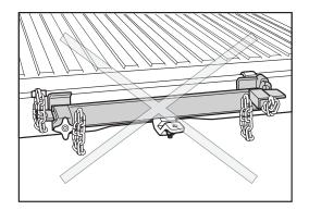
Weight-Distributing Hitch System – This type of system uses a "load-leveling" or "equalizing" hitch. The weight-distributing feature helps shift the trailer tongue weight to all the axles of the tow vehicle and the trailer axles.
