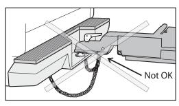
To avoid damage to the bumper and chains/cables when making a sharp turn, do not attach the chains/cables too close to the coupler. Consult your trailer manufacturer for the proper location of the chain/cable attachment to the trailer.
