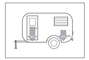
With this in mind, proper loading is extremely important. When loading a trailer, 60% of the total cargo weight should be positioned in the front portion of the trailer and 40% in the back. Then the load should be adjusted until the proper tongue load ratio is achieved.
