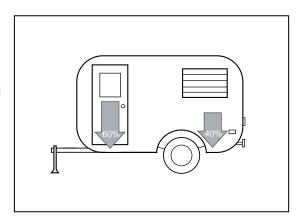
The trailer load should be balanced equally from side-to-side. Unequal side-to-side loading can negatively affect handling and braking. Once in place, all cargo should be firmly secured to prevent shifting. If the load should shift abruptly during braking or cornering, it could quickly affect the handling of your vehicle and cause a very unsafe situation.
