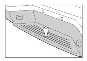
Receiver Hitch – A receiver hitch is bolted directly to the vehicle structure for added strength and durability. Infiniti bolt-on receiver hitches are designed specifically for Infiniti vehicles and include the necessary reinforcements, with ample clearance around bumpers, frame members, etc. These hitches allow for the removal of the ball mount when not towing.
