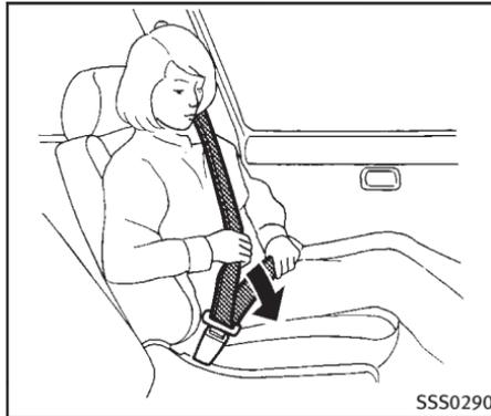
3. Position the lap belt portion **low and snug on the hips** as shown.
