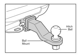
as the coupler on your trailer. Using a  $1^7/8$ " hitch ball in a 2" coupler, for example, could result in the trailer separating from the tow vehicle.
