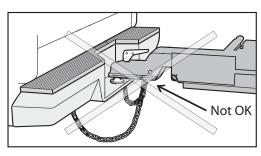
To avoid damage to the bumper and chains/cables when making a sharp turn, do not attach the chains/cables too close to the coupler. Consult your trailer manufacturer for the proper location of the chain/cable attachment to the trailer.
