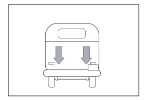
The trailer load should be balanced equally from side-to-side. Unequal side-to-side loading can negatively affect handling and braking. Once in place, all cargo should be firmly secured to prevent shifting. If the load should shift abruptly during braking or cornering, it could quickly affect the handling of your vehicle and cause a very unsafe situation.
