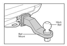
rating for the ball mount as well as the coupler on your trailer. Using a  $1^7/8$ " hitch ball in a 2" coupler, for example, could result in the trailer separating from the tow vehicle. The required hitch ball size is stamped on most trailer couplers.
